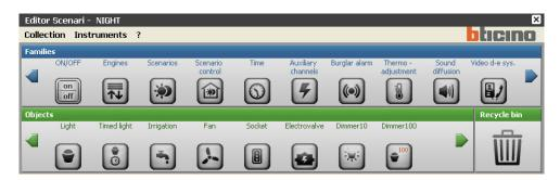
To configure a scenario, drag the object icons to the various fields below using the "drag and drop" function.
