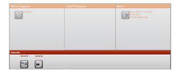
For example: The execution of the scenario will activate an instruction (General ON) to all actuators belonging to the ON/OFF family and an instruction (General OFF) to all actuators of the Motors Family.
